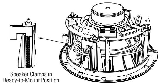
7. Insert the speaker straight into the mounting opening. Tighten the speaker clamp screws on the front of the speaker baffle. The speaker clamps will automatically rotate into position and begin clamping the speaker.
