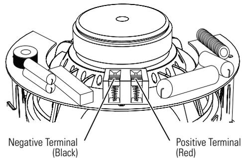
Press down on the terminal tab to open the hole; insert the bare end of the wire into the hole; and release the tab to secure the wire. NOTE: C283LP and C263LP models have post-type terminals. Press down on the post to open the hole; insert the bare end of the wire into the hole and release the post to secure the wire.
